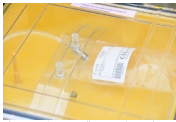
(f) Gas Sampling in a Tedlar Bag in the Sampling Box
