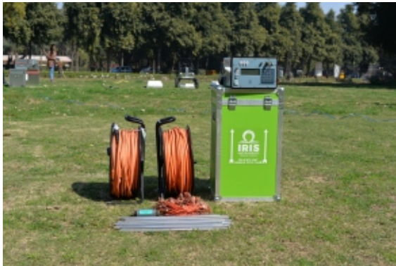
(a) Electrical Resistivity Imaging System: Resistivity meter, Electrodes, Cables and Connectors
