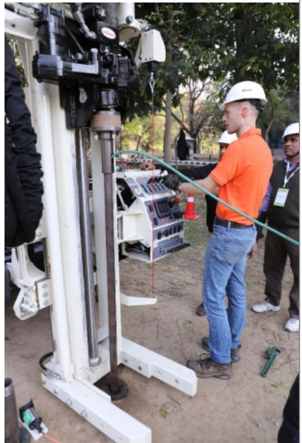
(f) Performing OIHPT test
