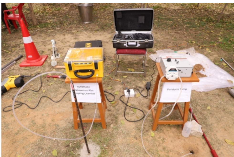
(g) GVP Tip attached with Vacuum Gas Sampling Chamber(Left) and Peristaltic Pump for Groundwater Sampling (Right)
