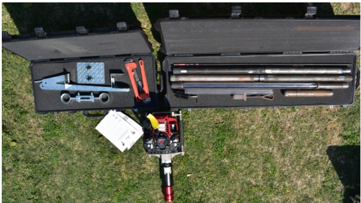
(e) Petrol Powered Core Sampling Kit with Hammer and Removal Foot Jack
