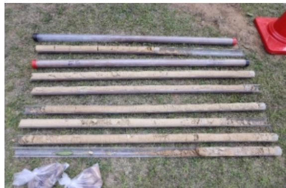
(h) Liners Containing Continuous Core Samples
