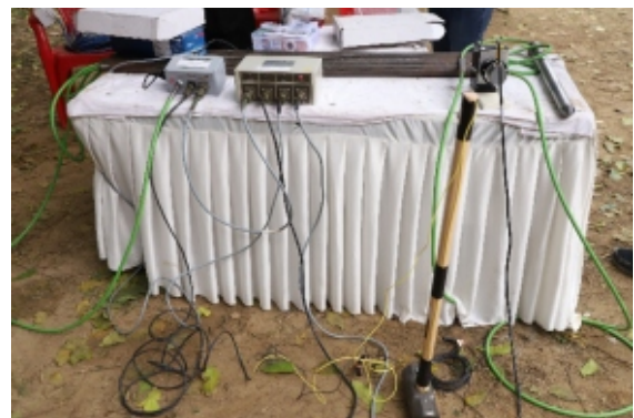
(h) Connecting Cone, CPT Controller and Laptop
